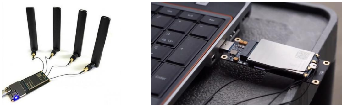
Figure 4 QUECTEL RM500Q modem used as COTS 5G NR UE device for the interoperability tests.
