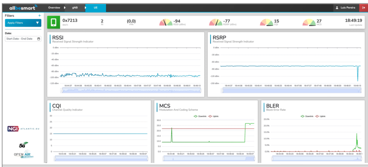
Figure 9 Visualization in real-time of PHY layers parameters for a specific UE.
